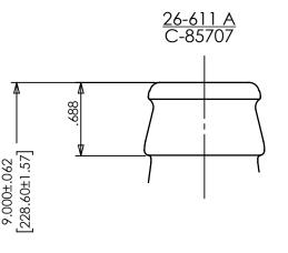
THIS BOTTLE IS DESIGNED TO PROVIDE CROWN REST CLEARANCE INDICATED ONLY. CUSTOMER MUST ADVISE IF ANY SPECIAL CLEARANCES ARE REQUIRED.
